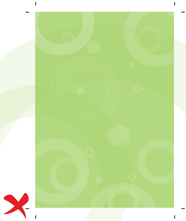
Incorrect file supplied with crop marks and no bleed
